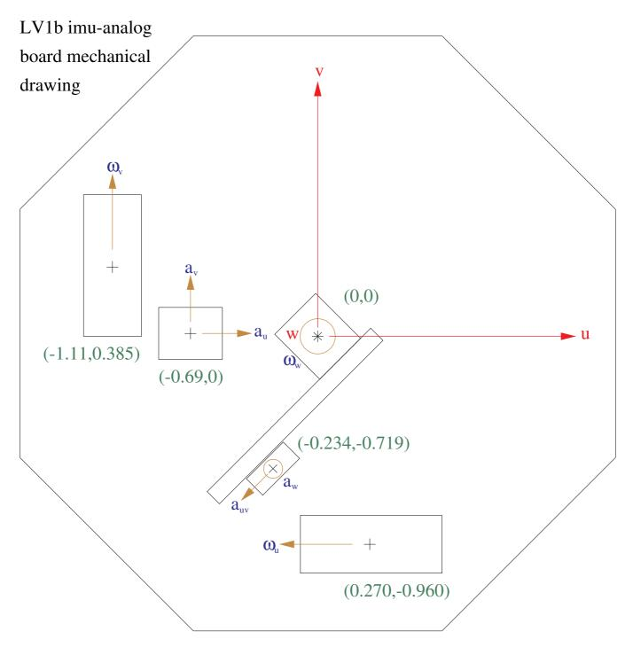
accelerometer arrows indicate the sensitive axis in the direction of positive output gyro arrows indicate the sensitive axis, positive output follows the right hand rule circles indicate the sensitive axis is up out of the plane of the drawing
