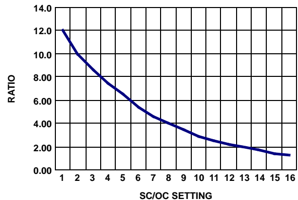
FIGURE 14. SHORT CIRCUIT TO OVERCURRENT RATIO
