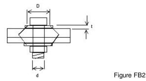
For the washers and each of the plates a separate stiffness value k is determined and the total stiffenss is determined in the same manner as springs in series. The equation for the individual frustrum is:
