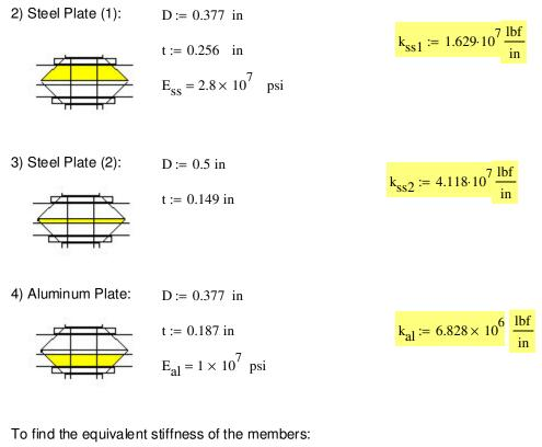
$$\frac{1}{k_{\text{mem}}} = \frac{1}{k_{\text{wash}}} + \frac{1}{k_{\text{ss1}}} + \frac{1}{k_{\text{ss2}}} + \frac{1}{k_{\text{al}}} + \frac{1}{k_{\text{wash}}}$$
