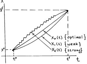
such that both  $\delta x$  and  $\delta x$  are small is called a weak variation, while a variation for which only  $\delta x$  is small is called a strong variation. Thus, conditions (2.2.6) and (2.2.7) can be used to determine a minimizing function x (t) only on the class of functions x(t) which represent weak variations of x(t). Another condition is needed to determine the minimizing function on the class of strong variations. Such a condition was developed by Weierstrass in the 1870's.
