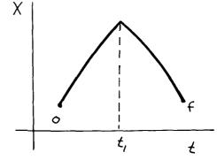
In developing the Euler conditions of Eqs. (2.2.31) and (2.2.12), it has been tacitly assumed that the derivative  $\dot{x}$  is continuous along the extremal arc, a condition that will not hold if the arc has corners (see preceding sketch) resulting from sudden control changes, etc. At a corner point, say  $t = t_1$ , the derivative  $\dot{x}$  is not defined. Hence, the functional J which is to be minimized is rewritten as
