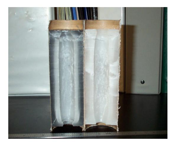
In both cases, this is this region of paraffin is in contact with the aluminum plug that is on the motor end of the spin caster. We will perform another test and see if this happens again. It may have something to do with the nature of the cooling of the grain near the plug or it may have to do with the disassembly of the grain holder after cooling has occured.
