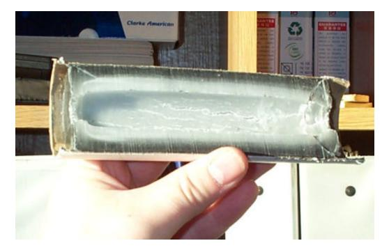
A second test was conducted to look at how the introduction of powdered graphite into the molten paraffin before spin casting would affect the final product.
