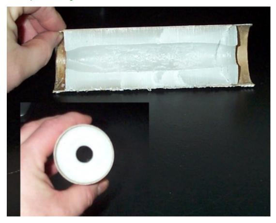
This first test was conducted specifically to see if a paraffin fuel grain could be spun-cast with the new apparatus. The initial volume measurement of the liquid paraffin is not exact because we didn't think to measure the height of the column of liquid paraffin before we sealed it up and put it in the spin caster. The 4.9 inches therefore is a estimate. (See calculations below)
