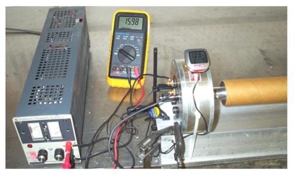
To verify that what we are reading on the new BC-500 tachometer is in fact an accurate representation of the RPM of the motor we did a slow speed, manual count of the revolutions over a one minute interval (measured with a stop watch).
