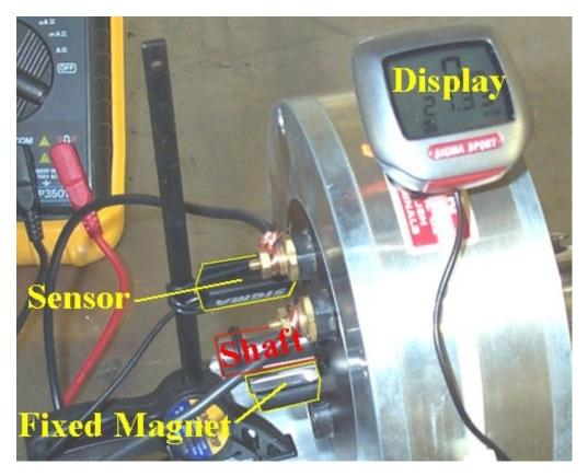
The problem with this bicycle computer is that it doesn't actually give you a RPM output, but instead it gives and mph or km/hr output. Though it is possible to map this velocity output to a RPM output. This is done by making the bicycle computer prompt you for a wheel circumference or "Wheel size" and then giving it the value of 1667. This number is a conversion factor that will cause the computers km/hr output to be the same as Revolutions per Minute. only scaled down by a factor of 10.
