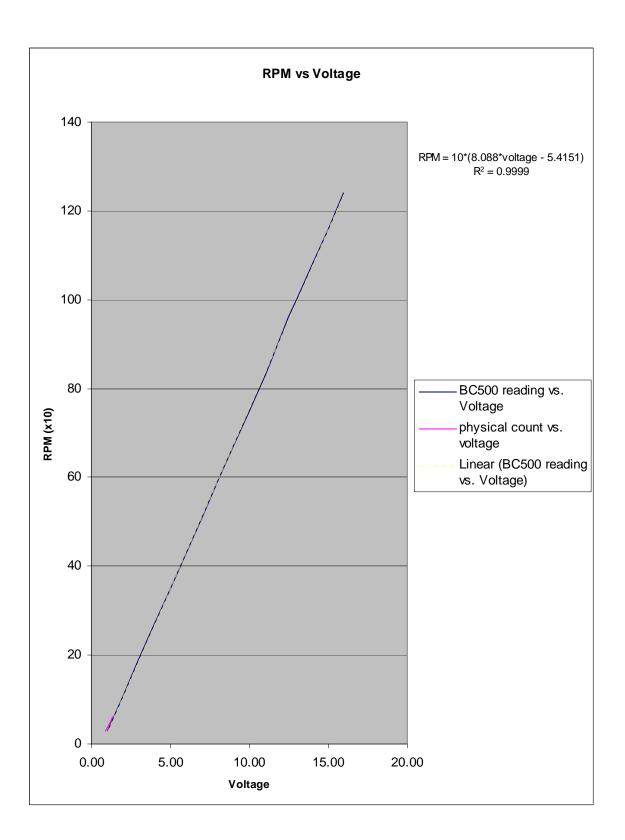
The procedure for altering the BC-500 is as follows:
